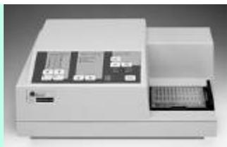
Read plates in a Plate Reader at the appropriate wavelength:
