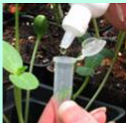
Add 10 drops of buffer (0.5 mL per leaf snap)
