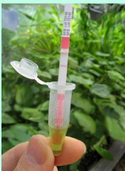
Add a test strip, wait 5 minutes
