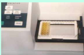
Read plates in a Plate Reader at 450 nm within 30 minutes of the addition of Stop Solution.
