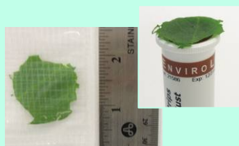
Leaf sample should be approx. 1" diameter, roughly the size of the canister cap
