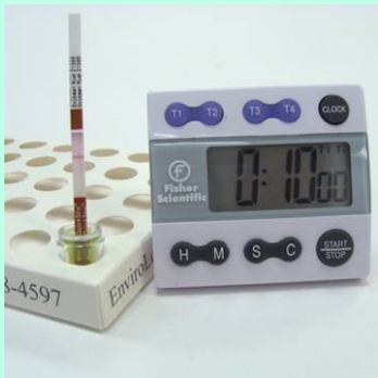
Add a test strip to the vial, wait 10 minutes
